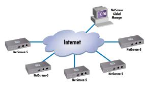
NetScreen-5 devices can easily be configured, managed, and monitored from a central site using a web browser, SNMP, Telnet, TFTP, CLI, or NetScreen Global Manager.
