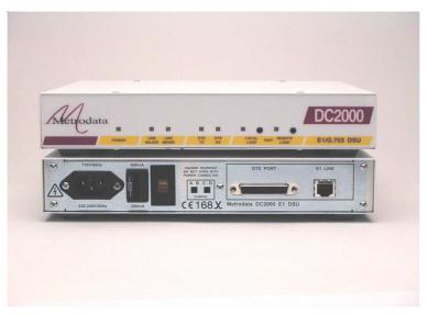
The DC2000 provides a new level of price/performance in connecting E1 G.703 2 Mbit/s leased lines to DTE equipment such as a router presenting an EIA-530, V.35 or X.21 interface. Data is carried on the E1 line as unstructured payload.
