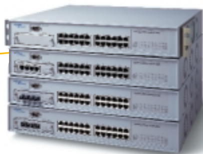
Figure 2: Business Policy Switch Stack.
