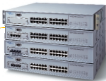
Figure 2: Business Policy Switch Stack.
