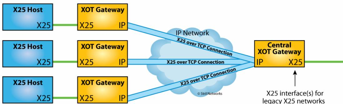
Several central gateways can be added to improve reliability by redundancy. Each Client XOT Gateway can have a list of Server XOT Gateways to use. If one Central XOT Gateway is unreachable, due to hardware failure or network problem, the next on the list is tried. Load sharing is done by rotating the list differently among the Clients. E.g. half of the clients prefer Gateway A as their primary and Gateway B as their backup, and the other half has Gateway B as their primary and A as backup.
