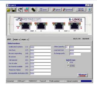
Each B-LinkU is supplied with a simple default configuration allowing you to plug and play. Intuitive Windows software supplied, allows you to easily configure and save any required changes. The software also provides access to the powerful protocol trace facility, which displays all messages transmitted and received on each line with user selectable filters for product test and development applications.
