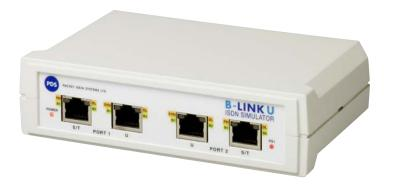
B-LinkU provides two ports with connection via S/T or U interface on each port.
