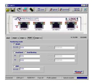
Each B-Link4 is supplied with a simple default configuration allowing you to plug and play. Intuitive Windows software supplied, allows you to easily configure and save any required changes. The software also provides access to the powerful protocol trace facility, which displays all messages transmitted and received on each line with user selectable filters for product test and development applications.
